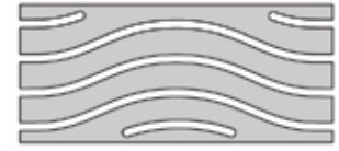
Type "W" Wave Grates. This is a top surface view. There are Cross Ribs underneath for support.
